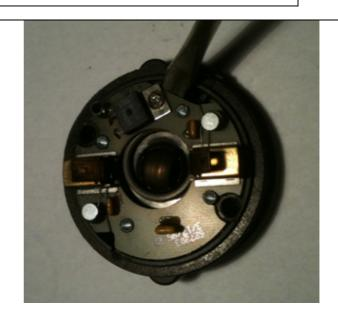
Use a 1/8" (3mm) drill to drill out the thermal switch rivet.
