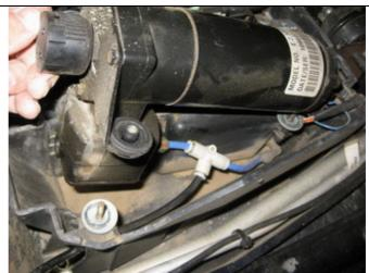
The Thermal Switch resides in the brush housing assembly, at the end of the motor. Remove the mount bracket and the 2 long bolts. Gently pry up the motor end, pry the wires out as well.
