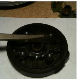
Clean the burrs from the end bell, screw the socket head screws into the holes drilled previously, they will cut their own threads. Start with your electric driver on low torque and slowly increase until just seated, or run in by hand.
